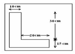
b) Find the moment of inertia of the lamina about x-axis shown in figure.8 M
